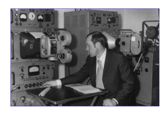
First Russian (Soviet) serial ionosonde AIS-56. It was installed in Tomsk in 1957 and has operated continuously for almost 40 years (1957-1996).
