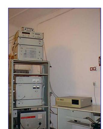
Digital ionosonde Parus (designed and built at IZMIRAN), operating in Tomsk since 1996.
